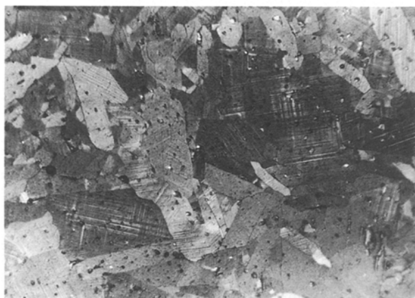
Figure 4 Optical microstructure of electrochemically textured sample (F + Seed) ( \times 500 ).
